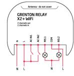
The device without a target configuration loaded via Object Manager tool, has the minimal embedded configuration. The in-puts are connected to the outputs, which allows for local loads control.
