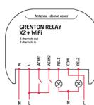
The device without a target configuration loaded via Object Manager tool, has the minimal embedded configuration. The inputs are connected to the outputs, which allows for local loads
