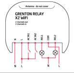
The device without a tar-get configuration loaded via Object Manager tool, has the minimal embedded con-figuration. The inputs are connected to the outputs, which allows for local loads control control.
