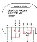
The device without a target configuration loaded via Object Manager tool, has the minimal embedded configuration. The inputs are connected to the outputs, which allows for local blind control.
