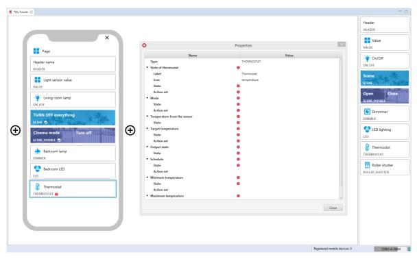
For thermostats, ready-made templates for the THERMOSTAT widget are defined. To add a THERMOSTAT widget with a ready template, drag the virtual thermostat from the list of objects to the interface page:
